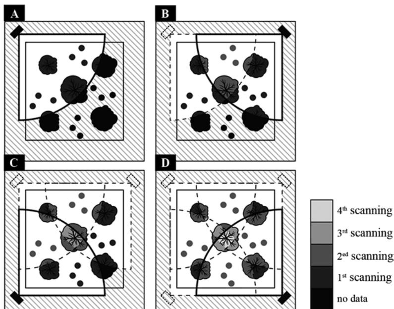
**Fig. 3.** Principles of registering point clouds measured from different locations and georeferencing point clouds passing through a registration process.
