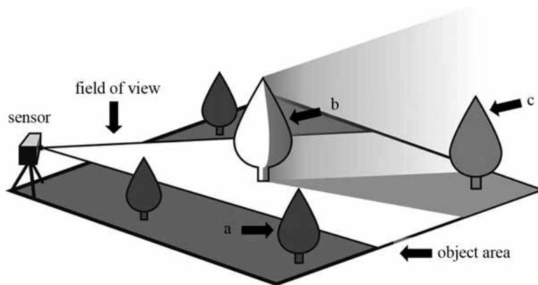
**Fig. 2.** The 3 types of occlusion problems: (a) view occlusion; (b) self occlusion; and (c) ambient occlusion.
