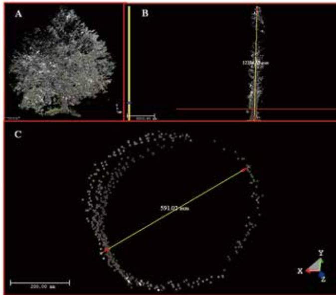
**Fig. 4. A. Using LiDAR data to extract stumpage; B. using LiDAR data to measure tree height; C. using LiDAR data to measure diameter at breast height.**
