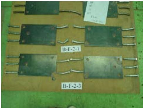
Fig. 9. Failure of flat-type metal connectors assembled with 2 bolts on a beam member.
